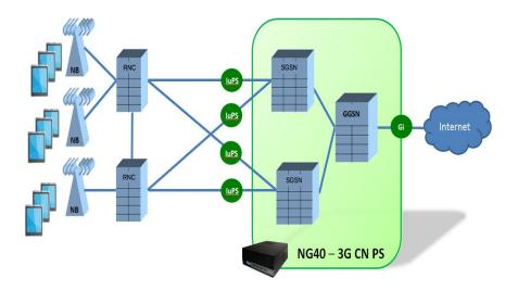
DEMONSTRATION TEST Core Network (CN) emulator for multiple SGSNs with Control Plane and User Plane functionality over Ethernet
