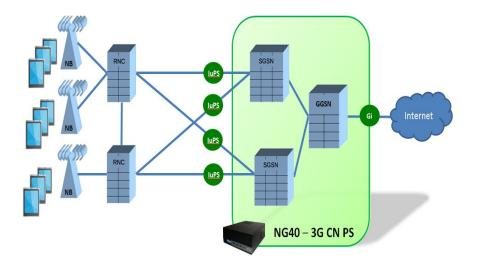
FUNCTIONAL TEST Core Network (CN) emulator for multiple SGSNs with Control Plane and User Plane functionality over Ethernet
